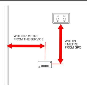
Note: Controller must be mounted away from any moisture or potential water splashing.
